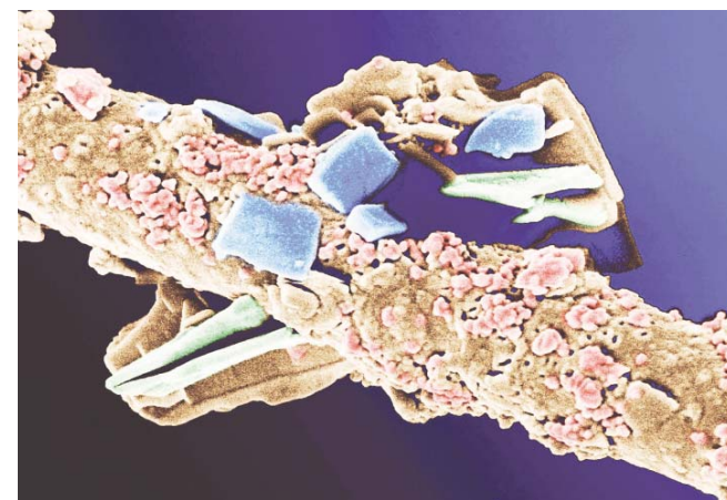
FIGURE 5. Nanoparticles on a strand of filter fibre. © LENNART NILSSON PHOTOGRAPHY AB/CAMFIL AB
