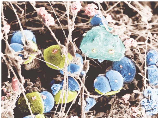
FIGURE 1. Pollen and combustion products trapped in an air filter. © LENNART NILSSON PHOTOGRAPHY AB/CAMFIL AB
