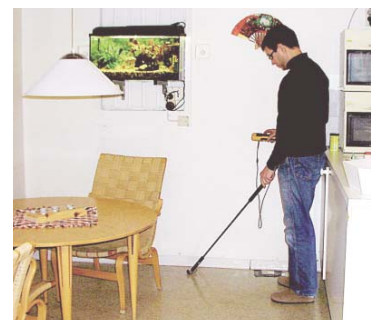
FIGURE 9. An inventory carried out before rebuilding will reveal critical construction solutions and faulty functions that could constitute risks for the indoor environment and the air quality. This means that major problems can be discovered in time, with great cost savings as a result. The photograph shows moisture measurements being carried out with a moisture meter, to find floor areas with excess moisture content. If floor coverings are placed on top of damp floors, chemical substances could be released and affect the quality of the air.
