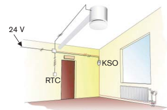
FIGURE 13. An active ATD with an external room thermostat and sequentially controlled radiator valves.
